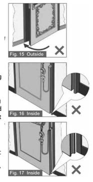
B. On the doors and frames that have a narrow gap, pull out the soft sleeve before the door is completely closed, otherwise the soft sleeve may get stuck in the gap.
